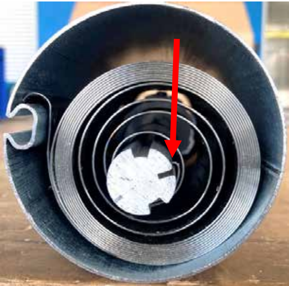
Good spring in roller tube
