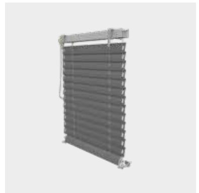
DIPLOMAT 50 Cable-suspended standard external blind with 50 mm aluminium slats. Max. width 3500 mm Max. height 2700 mm
