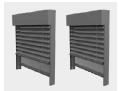
SKY-MULTI PELMET IR SKY-MULTI PLASTERED PELMET IR Pelmet screen / plaster base variants with integrated insect screen roller blind. Max. width 1800 mm Max. height 2500 mm
